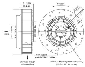
Lead wire spec. AWG24 UL3266 Color (+) Red (-) Black (sensor) Yellow
