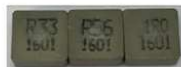
Ps: Spray printing effect : can be accepted if recognizable
